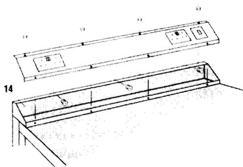
1. Undo screws to remove front of service panel.
