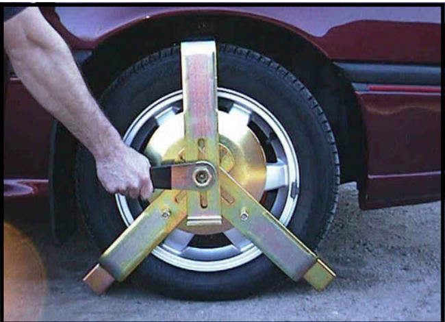
9. Using spanner provided tighten nut in a clockwise direction until it locks up solid.
