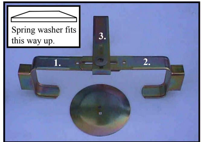
**2.** Position lower arms as shown and lay top arm on top. Place in position spring washer, push square head of M12 x 40mm coach bolt into round disc. (Tap with hammer if tight fit) until dome head touches disc. Offer up round disc to lower arm, ensure that the pressed dimple on the disc locates securely in slot in arm, this is to prevent turning.
