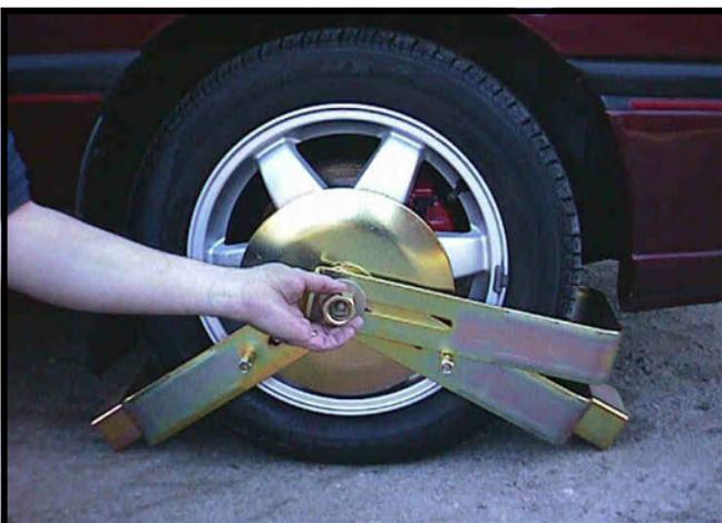
**5.** With left hand lift nut and disc assembly to centre of wheel.
