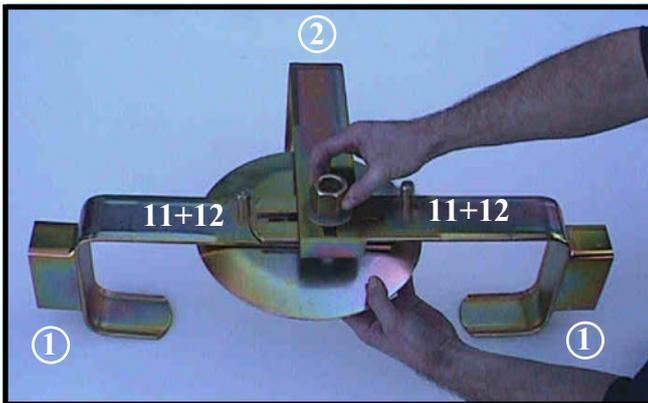
**3.** Insert key and turn  $\frac{1}{4}$  turn anti clockwise to remove hollow nut from inside cover plate and screw on finger tight but still allowing arms to slide freely. Please ensure that the recess on back of nut is located into hole in large spring washer.
