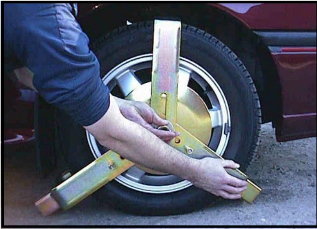
7. Still holding up nut with left hand pull the right wheel clamp arm in tightly to tyre.
