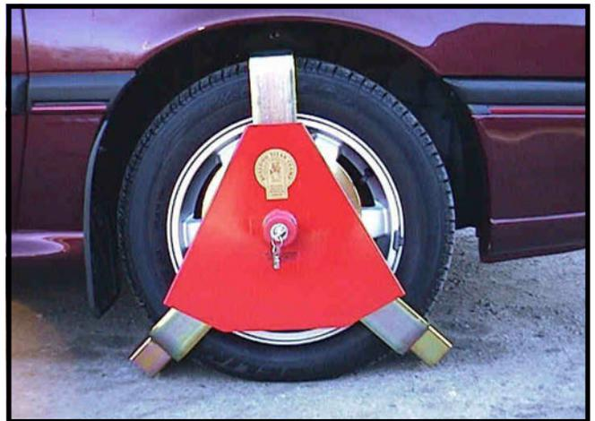
10. Ensure lock bolt is unlocked (key inserted and turned 1/4 turn anti-clockwise). Now locate tube on back of red cover over the hollow nut, then turn key 1/4 turn clockwise to lock. Note. To prevent lock bolt from turning when key is operated press thumb against the face of the red plastic cap. To Un-Lock. Insert key, rotate 1/4 turn anti-clockwise, remove Cover plate, reverse steps 9 back to 5.
