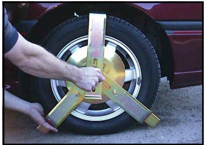
8. At this point hold up nut with right hand and pull left wheel clamp arm in tightly to tyre. Now tighten nut.
