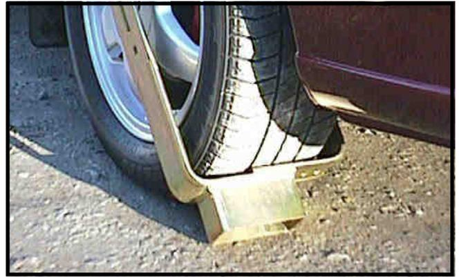
**2a.** Make up each arm and arm return to width of tyre (allow for width of disc, part no. 6).
