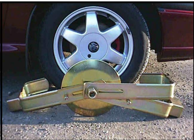
**5.** Push extended clamp arm assembly around base of wheel as shown.
