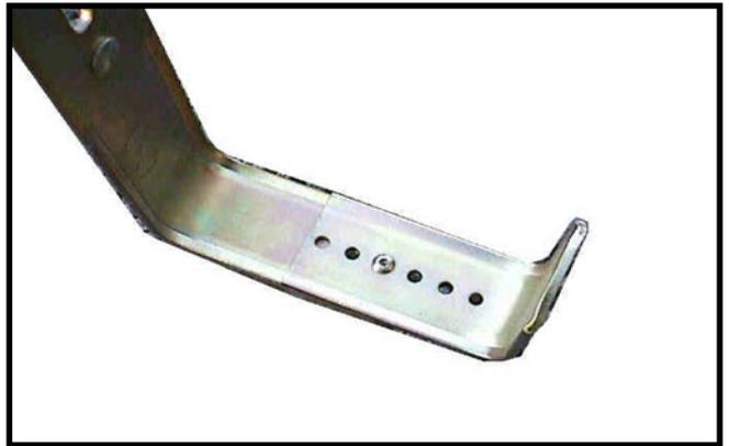
**2b.** Insert one M8x12mm button head screw at this point. You may have to finally adjust width of one or more arms on final assembly. NB: fit remaining screws in each arm only after clamp has been fitted and removed. Tighten with allen key provided. Tap aluminium plug into head of screw. These can be removed with a drill when readjustment is required.
