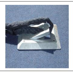
The Motorcycle Locking Loop - Bolt Down is ideal for securing motorcycles. The Loop is bolted onto the ground providing a very high level of security when used with the motorcyclists own locking chain. The lock loop is designed so it can be operated with gloves on and when not in use presents only a minimal trip hazard (The unit is only 20mm above ground). 4 x high security shear nuts and bolts are supplied for installation.
