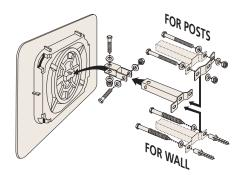
Supplied complete with bolts and brackets kit, adaptable for walls or for posts 60 to 90mm in diameter. Kit is robust, tested to withstand winds of up to 183km/h. Easy to install, allowing precise adjustment of the position of the
