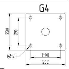
Bolt down/flanged products are supplied with a base plate(s).
