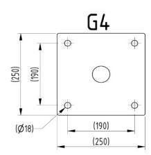
Bolt down/flanged products are supplied with a base plate(s).
