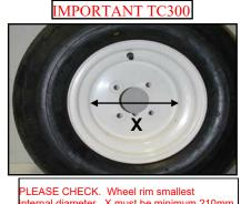
ternal diameter. X must be minimum 210mm
