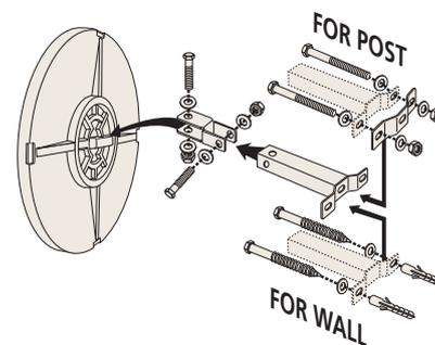
Supplied complete with bolts and brackets kit, adaptable for walls or for posts 60 to 90mm in diameter. Kit is robust, tested to withstand winds of up to 183km/h. Easy to install, allowing precise adjustment of the position of the mirror.
